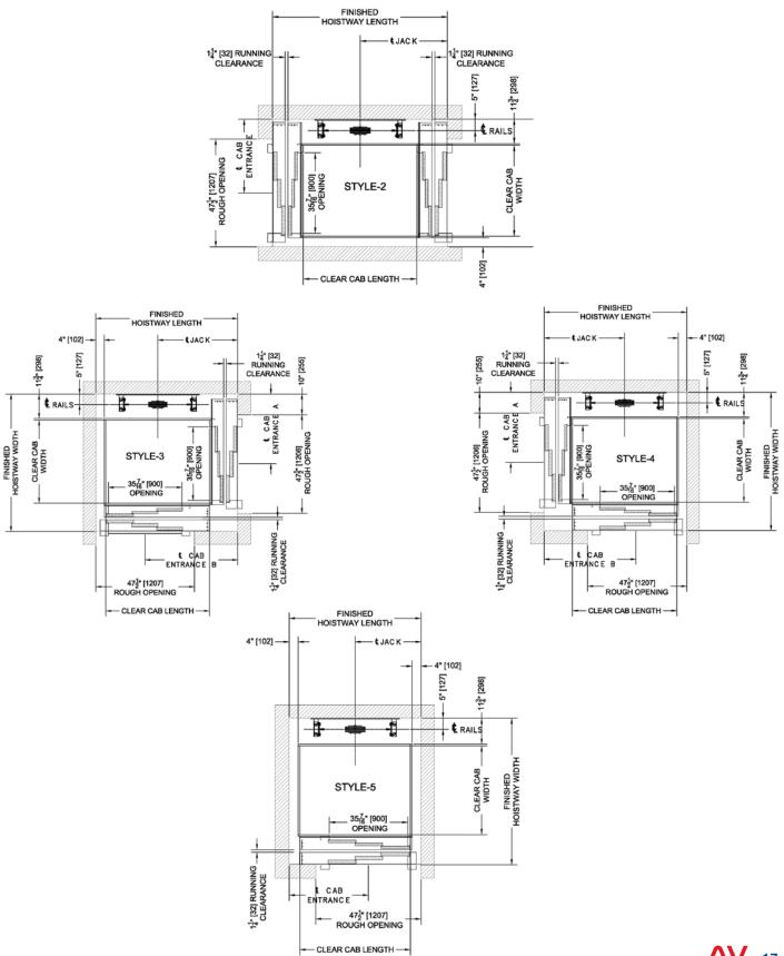
Premium Door Package - sliding elevator hall door with tandem sliding elevator car door
