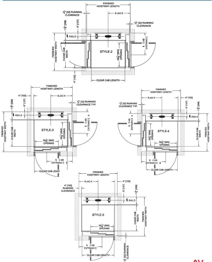
Upgrade Door Package - swinging hall door with sliding elevator car door
