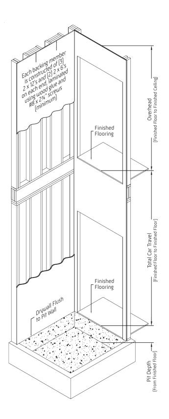
Each backing member is constructed of (3) 2 x 12's and (2) 2 x 6's on each end, laminated using wood glue and  $\#8 \times 2\%$ " screws (minimum).
